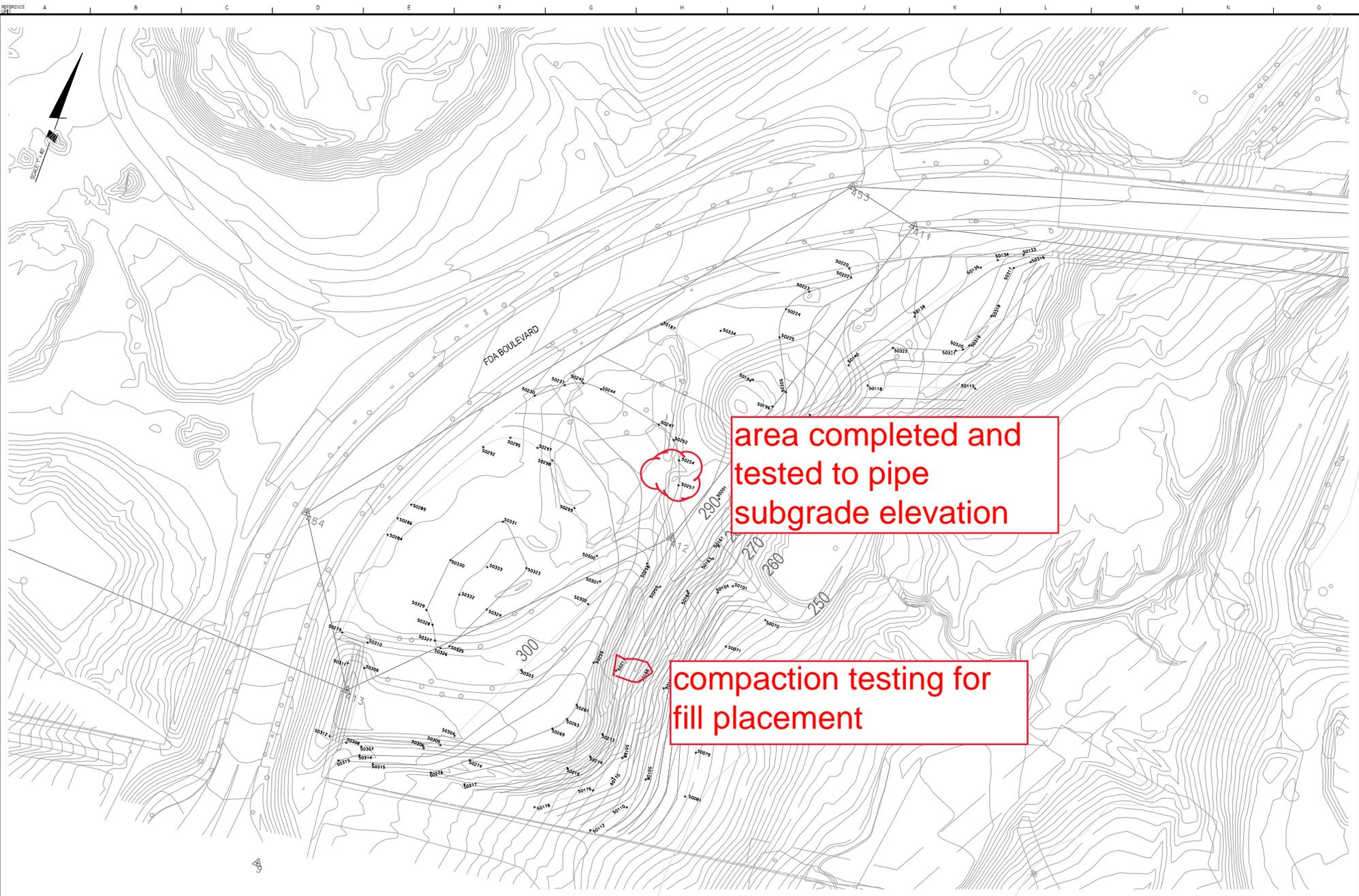
area completed and tested to pipe subgrade elevation
